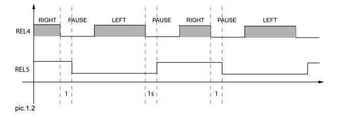
$SF81 \rightarrow 2 \rightarrow REL4$  and REL5 carries out the functions, which illustrate the chart. SF75 TL - time relay attach turnover LEFT (default = 10sek.) SF76 TR - time relay attach turnover RIGHT (default = 10sek.) SF77 Tp - pause time (default = 20sek)
