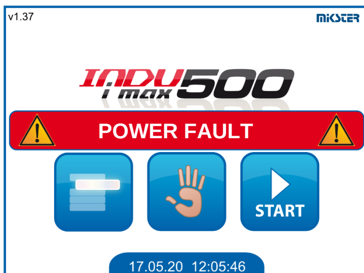
Screen after a power failure occurs that interrupts the program
