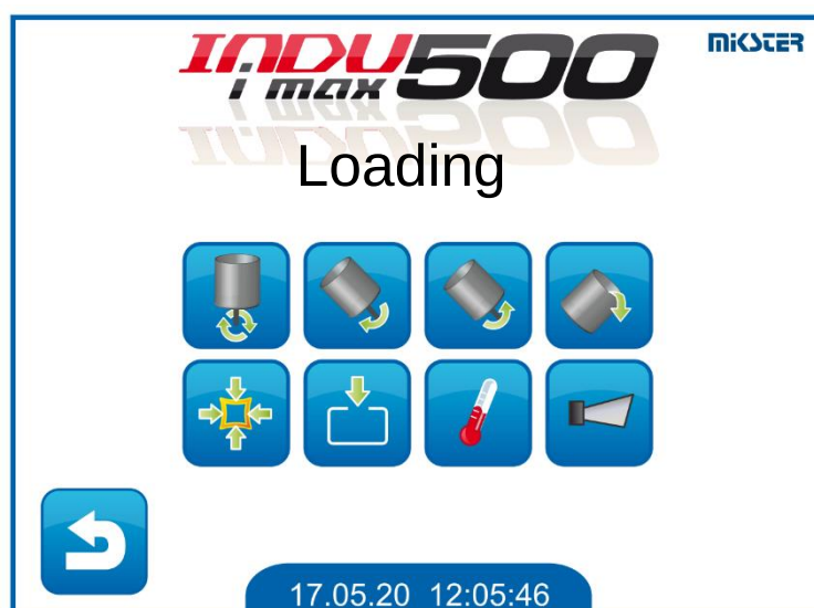
Screen for selecting active relays during loading or unloading
