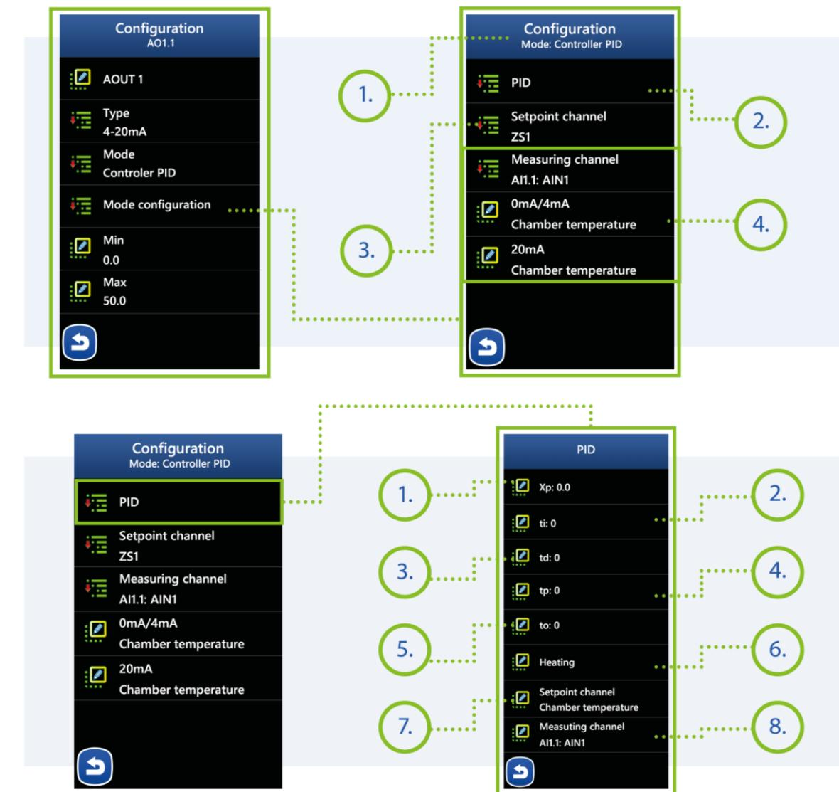
Menu | Service functions | Inputs/Outputs | Analog outputs | Configuration
