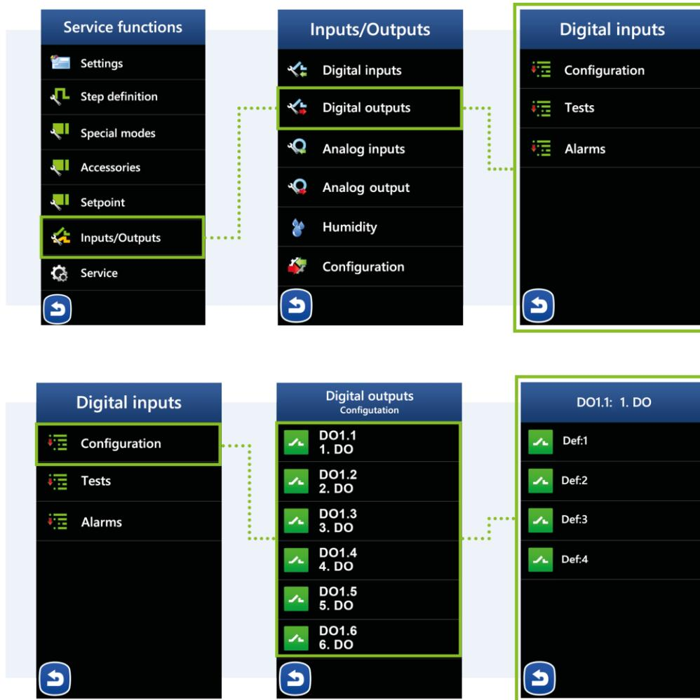
Menu | Service functions | Inputs/Outputs | Digital Outputs | Configuration
