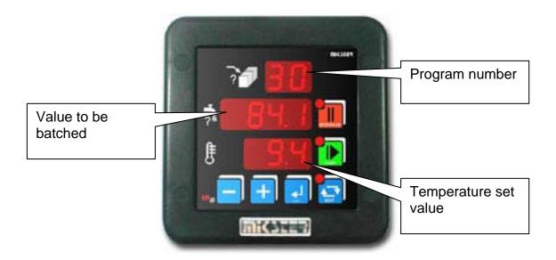
The control is destined for batching of arbitrary volumes of arbitrary medium at set temperature. Particular emphasis has been put to ensure proper operation in most harsh environmental conditions.
