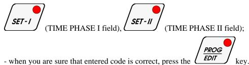
When the code is correct, the unit switches to programming. The displays will show parameters of a program, number of which is displayed in the PROGRAM field.
