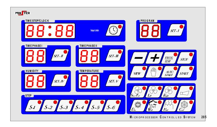
All information regarding the operation mode of the "MIKSTER MCC 026" (in-operation state, values of preset and read out parameters, equipment on / of signalling) is displayed on numeric displays and signalled by diodes. If particular unit is in operation or given function is active, the diode is continuously on. Blinking diode indicates waiting state or signals instantaneous value.
